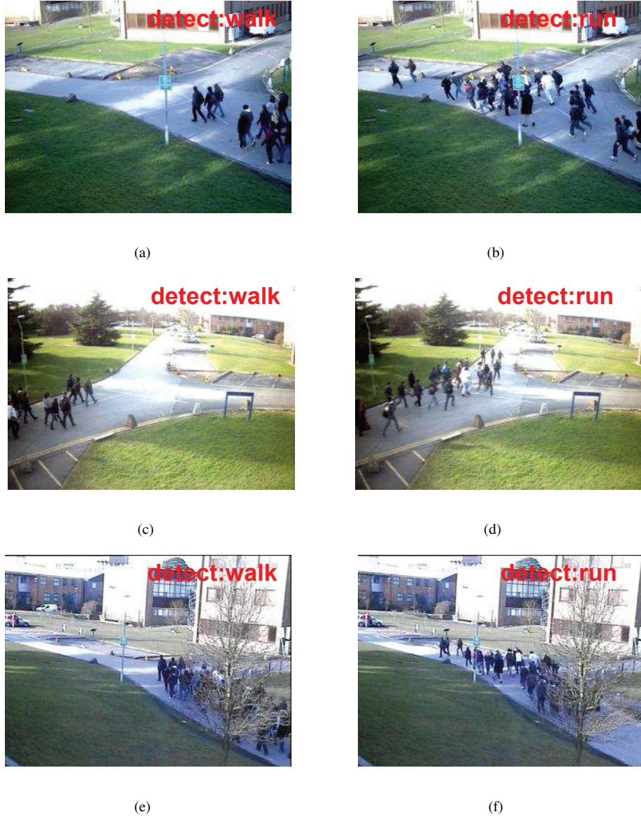
Fig. 6: Detection results of the normal and abnormal scenes of Time 14-16 captured by the distributed camera network, the individuals are moving from right to left. (a)(c)(e): The detection result of one normal frame, the individuals are walking in one direction. (b)(d)(f): The detection result of one abnormal frame, the individuals are running in one direction.
