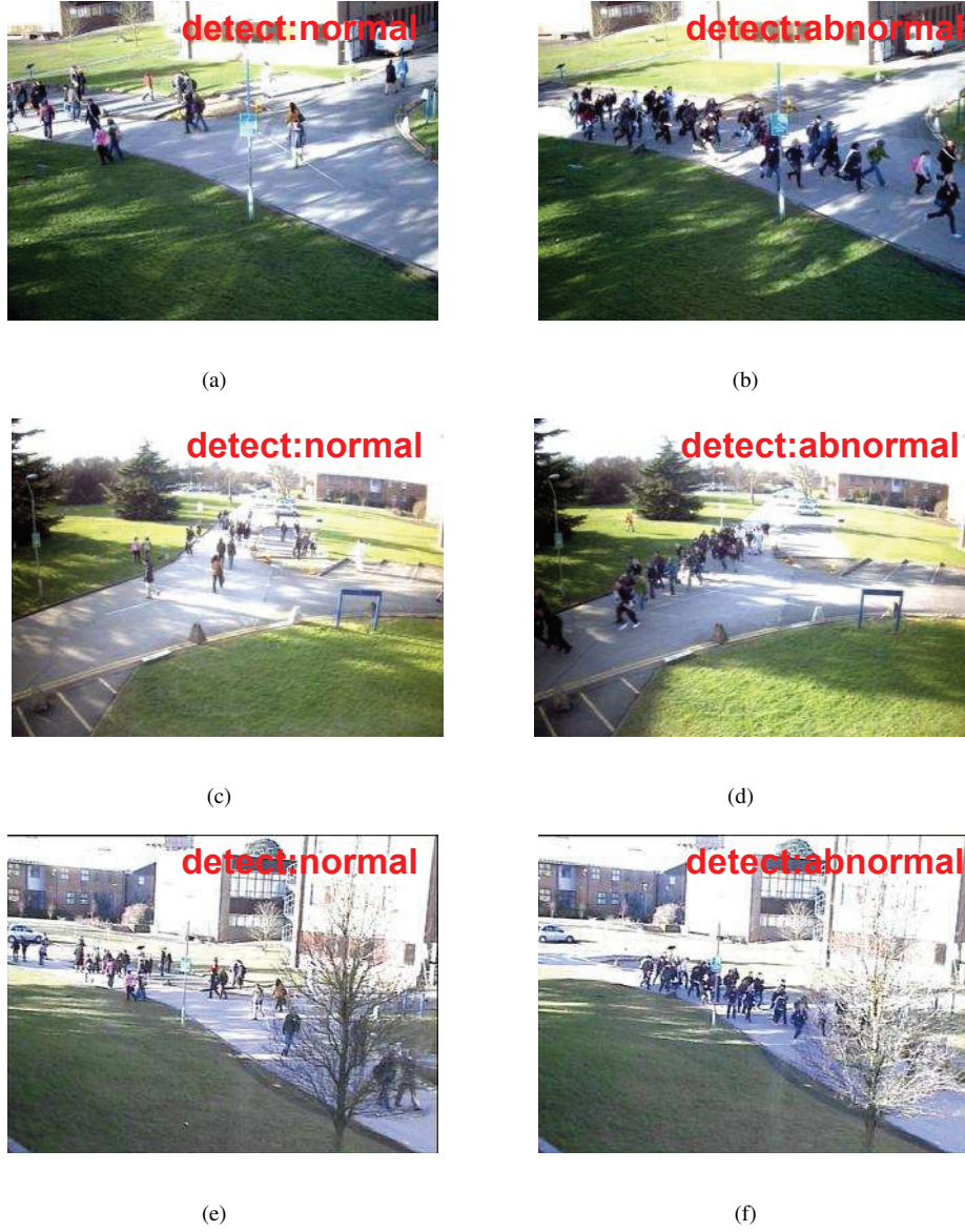
Fig. 4: Detection results of the normal and abnormal scenes of Time 14-17 captured by distributed camera network. (a)(c)(e): The detection result of one normal frame. (b)(d)(f): The detection result of one abnormal frame.
