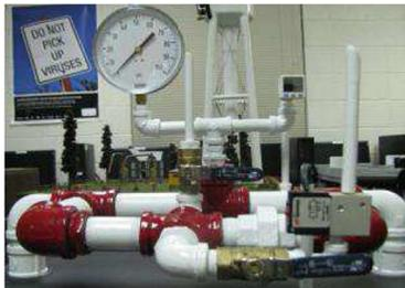
**Fig. 2.** Gas pipeline testbed
